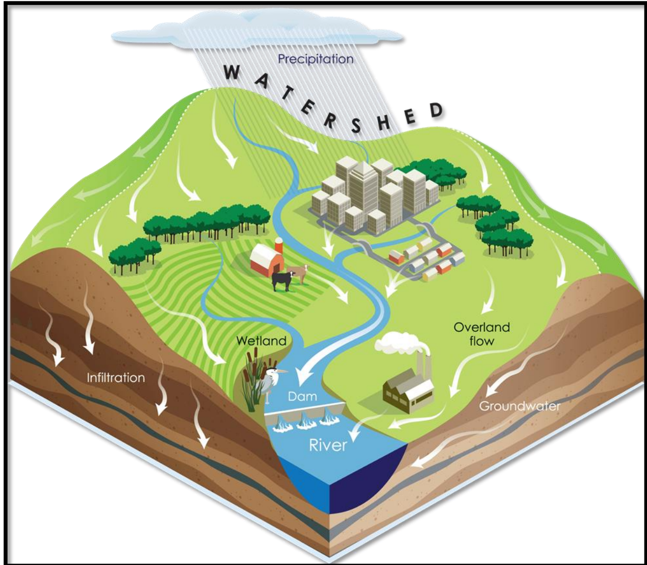
Figure 1-3. Watershed graphic illustration of stormwater runoff courtesy of Lake County Illinois Stormwater Management Commission.
